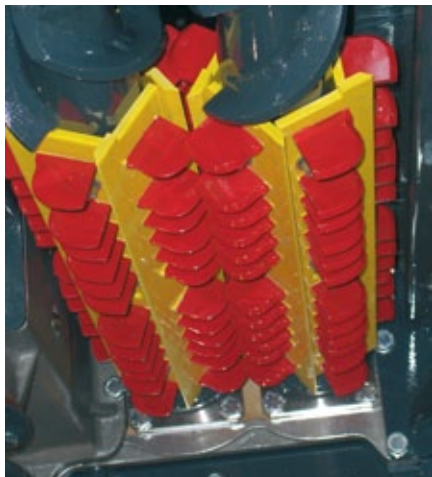
ROTO CROSS CUT slices the stalk vertically to get better decomposition.
